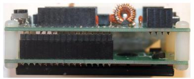
The combined 16-way plug and socket when mated together, have a height of a little under 12mm. Therefore it is necessary to have a gap somewhere.
