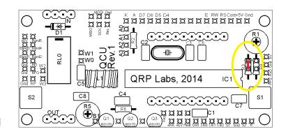
6) Install two 16-way connectors on the main PCB and LCD.
