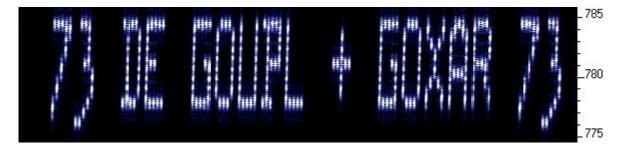
The following image shows part of the same thing in Argo's 3 second "slow" mode. The larger fourier transform bucket size means the image is more clear, but the faster scroll rate makes the letter's height to width ratio somewhat less attractive. Other slow-speed fourier transform software present more
