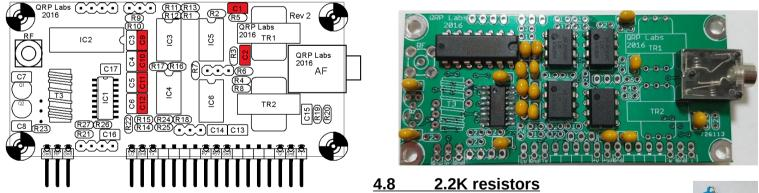
These are the 12 resistors R1, R2, R3, R4, R5, R6, R7, R8, R12, R13, R17 and R18. The colour code is: red-red-black-brown-brown. All of the resistors in this kit are installed vertically. So you need to bend the wires over very resistor as in this picture (right).
