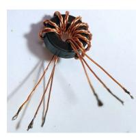
Now use a DVM to test for continuity. Re-arrange the wires so that there is continuity from A-A, B-B, and C-C in this photo.
