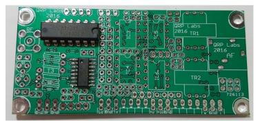
opposite diagonal ends of the chip. Then you can check that the chip is nicely seated on the board before soldering all the other pins. It is easy to make adjustments when only two pins are soldered, by re-heating the joints. But you cannot do that when you have 16 pins soldered! When you're happy with the position of the IC, solder all the other pins.
