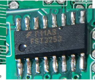
necessary corrections. When you are happy with the chip position, you can proceed to soldering the other pins. Pay particular attention to pin 8, which is connected to ground. Although the pad is connected to the groundplane with thin thermal traces, it will still tend to dissipate heat away from the joint, which can make it harder to get a good joint.
