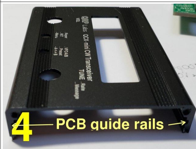
4 Here's the top half of the enclosure. Note the PCB guide rails in the extrusion walls.
