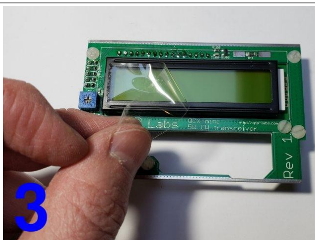
3 Peel off the plastic protective coating from the LCD module.
