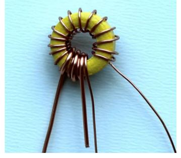
transformers T1 and T2. Note how they are a mirror image of each other, so that they neatly fit the board. As I said, this is not strictly necessary – it just makes things easier and neater!
