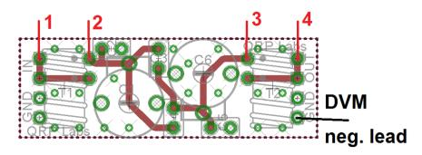
on one of the ground pins, and hold the positive probe to each of the points labelled 1-4 in this diagram. You should measure 0 ohms in every case! If you do not – then it means you have either connected something wrongly, or have not properly scraped/burnt off the enamel wire insulation! So go back and check everything!
