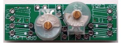
When soldering the pins, try to be FAST. You don't want to risk melting the plastic of the capacitor insulation and body.
