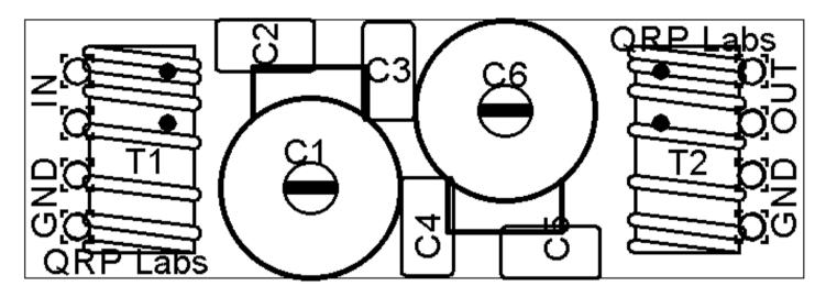
The PCB is quite small and the parts are close together. You are recommended to use a low wattage iron with a fine tip, and fine solder e.g. 1mm diameter or less. Take care not to overheat the PCB and risk damaging it. A well-lit area and magnifying glass may assist. Be careful not to bridge solder across closely-packed connections. I recommend checking with a DVM to make sure no solder bridges have been inadvertently created. Take care to ensure correct alignment of the 4-pin plugs.
