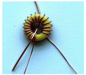
The photo (right) shows the completed second winding (thick wire). There are THREE turns in the 15m BPF. Check the number of turns required, for the band you are building (see parts list). Remember
