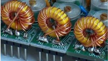
winding), and also the thick wire (coupling winding) if you decide to solder it in the hole, rather than direct to the pins.
