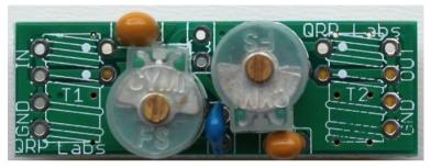
The coupling capacitor between the two tuned circuits is made up of two positions on the board, C3 and C4. This is because for some bands, the capacitance is made up of two smaller capacitors in parallel. In the photograph, the coupling capacitor is the blue one in this case (this is the 15m filter).
