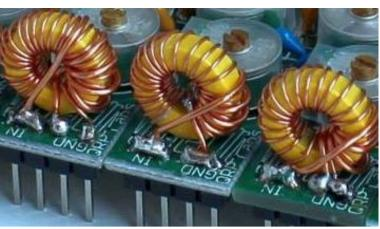
Do not solder the "hot" (non-ground) end of the main toroid windings yet! This will be done temporarily first before installation in the PCB hole – see "Adjustment" step, below.
