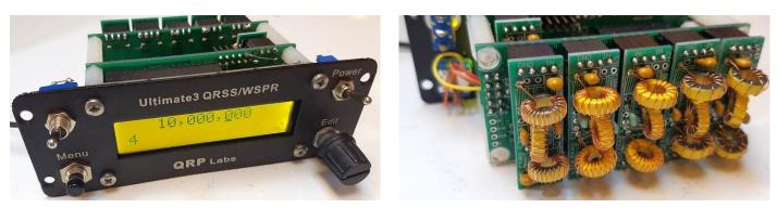
The 60m band LPF filter is plugged into the socket on the main VFO/SigGen board; the other LPFs 40, 30, 20, 15 and 10m are plugged into the relay board. The display is configured simply
